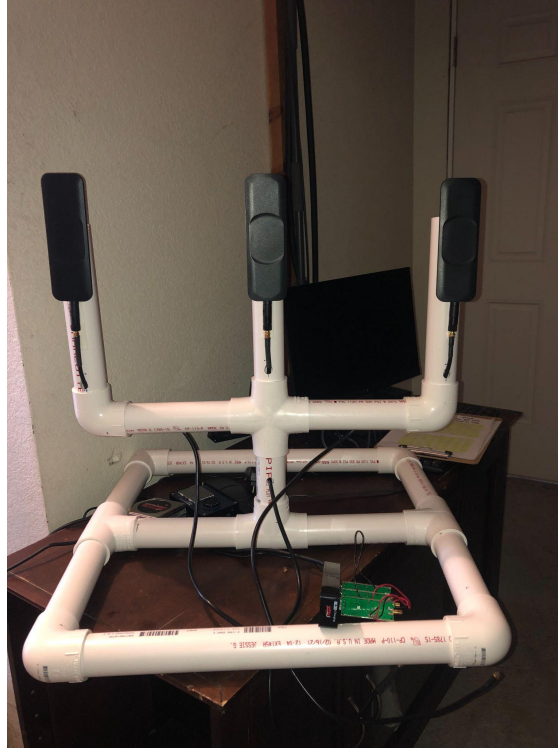
Figure 43 - Final 3 Antenna Array (3AA)
